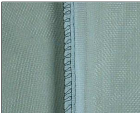
Overlock sewn joint with 3 needle for extra strength
